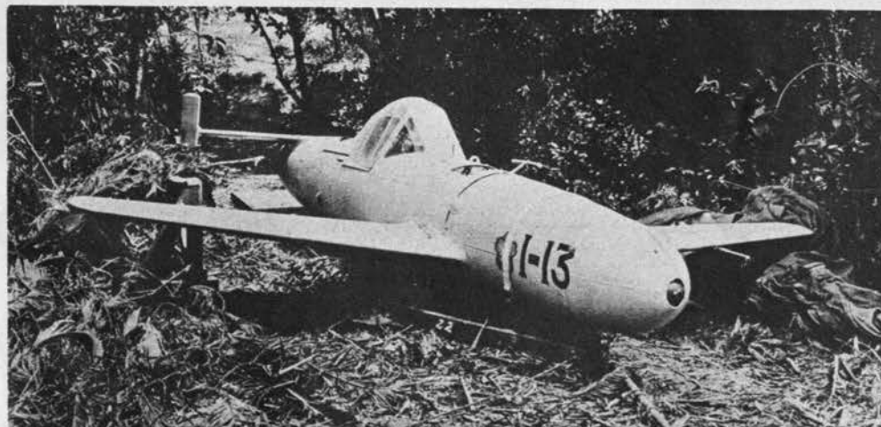
Baka's fins and rudders can be seen on either side of parent Betty's fuselage (top). Lower picture shows the prominent canopy. Note the simple ring and post sight atop the fuselage.
